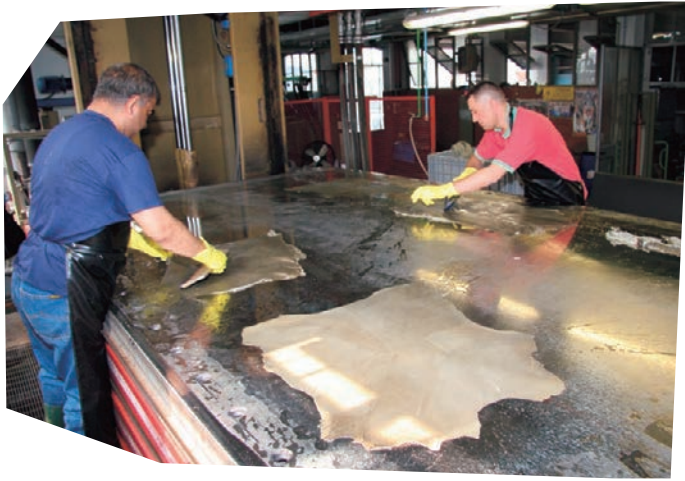
Figure 2–10: Vacuum-drying some suede skins.
