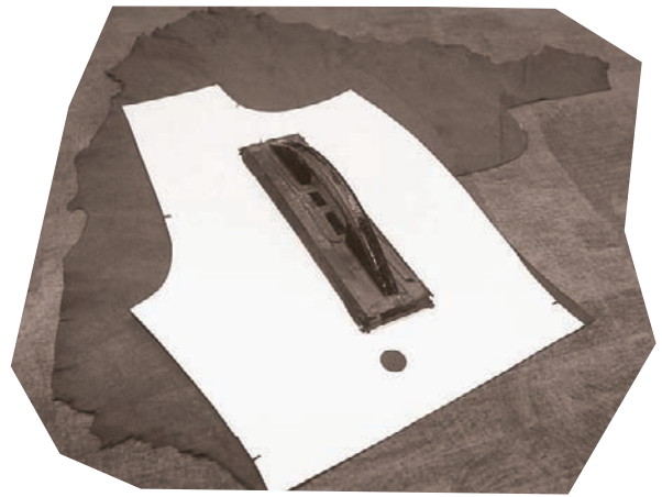
Figure 6-5: Using a weight to hold down a pattern while cutting.
