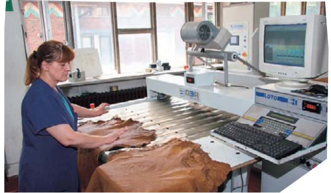
Figure 2–18: A skin measuring machine.
