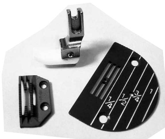
Figure 7-4: Teflon® teeth, foot, and plate.
