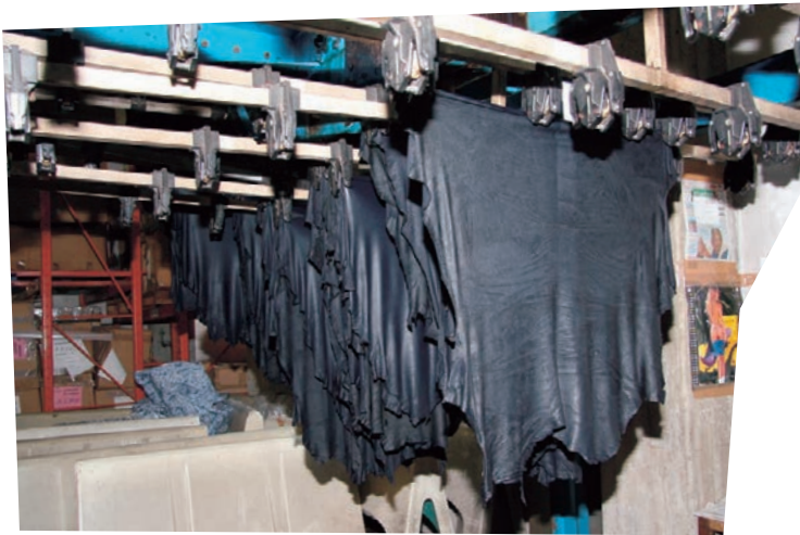
Figure 2–11: Air-drying dyed nappa skins.
