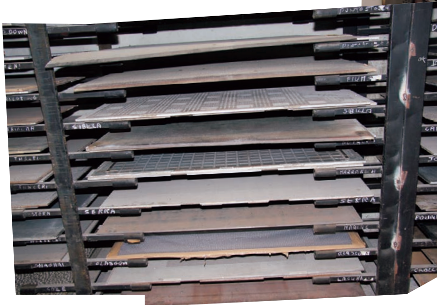
Figure 2–22: Embossing plates, used to produce a patterned skin.
