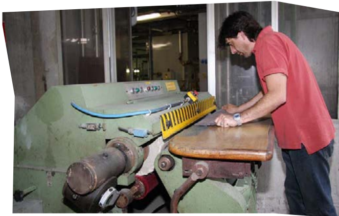
Figure 2–14: A suede polishing machine.
