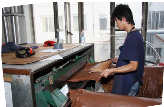
Figure 2–15: A suede de-dusting machine.
