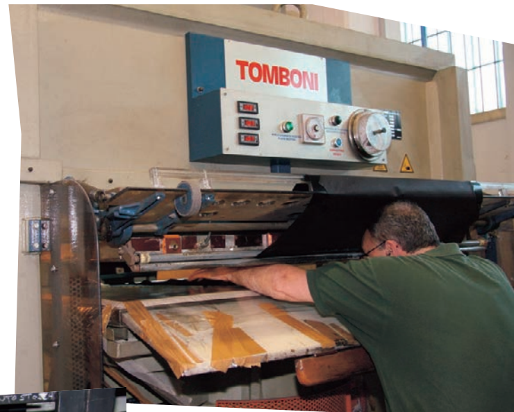
Figure 2–23: An embossing machine.
