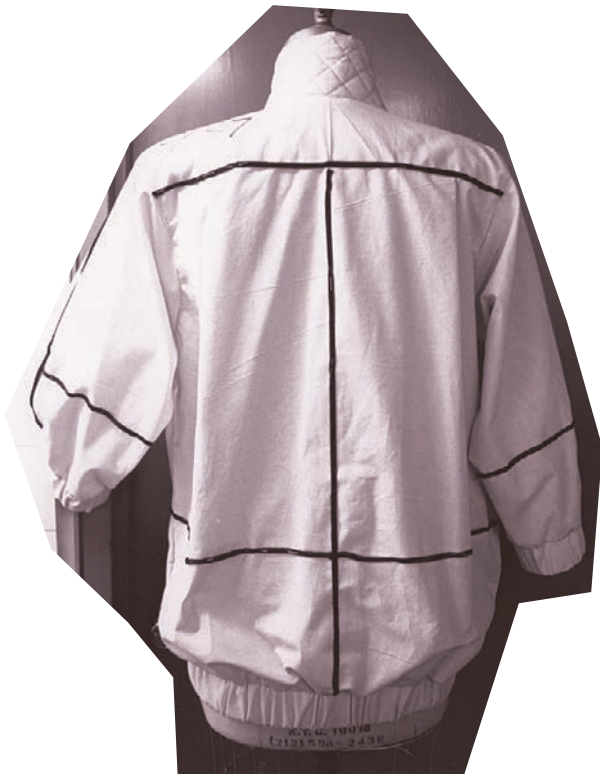
Figure 4-3: Back of a muslin showing styling tape to denote cuts.
