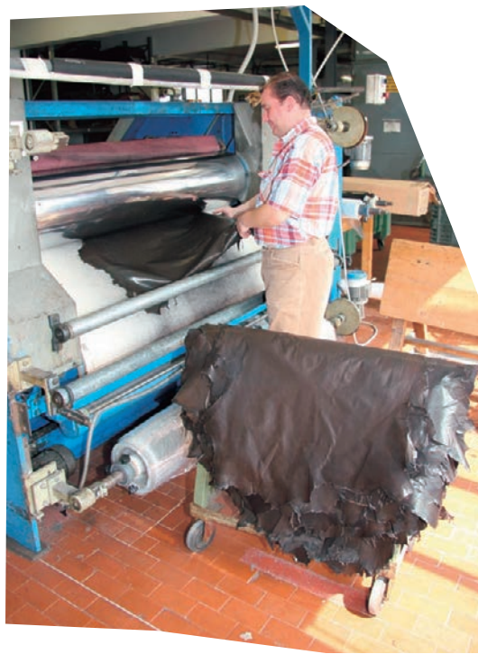
Figure 2–16: An ironing machine.
